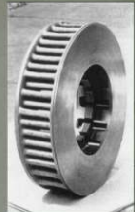
Fig: Cast brake disk particle of reinforced aluminum.
